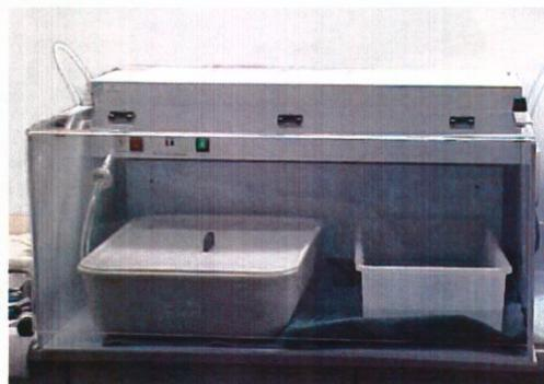
Ventilation cabinet to contain and capture vapors during endoscope reprocessing
