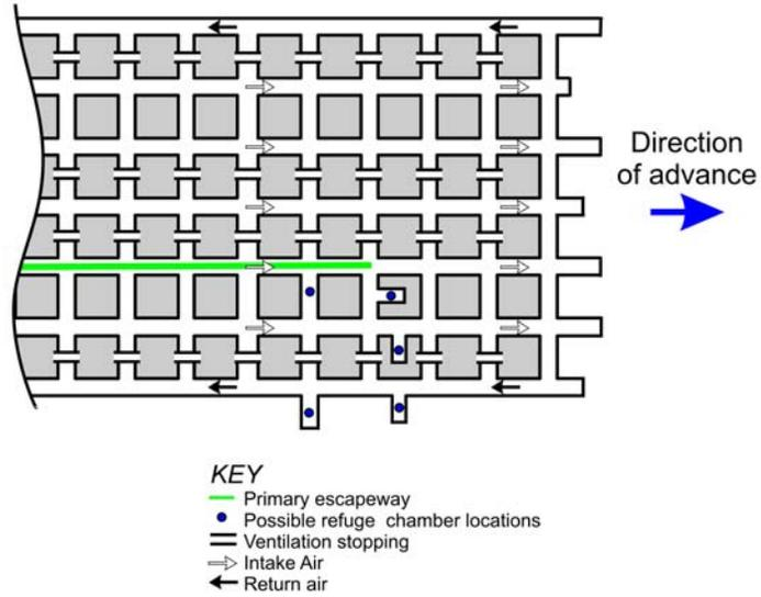
Figure 3 – Possible locations for refuge chambers in a development heading. The main options are a cross-cut or a stub entry. Note that a stub entry would require proper ventilation.
