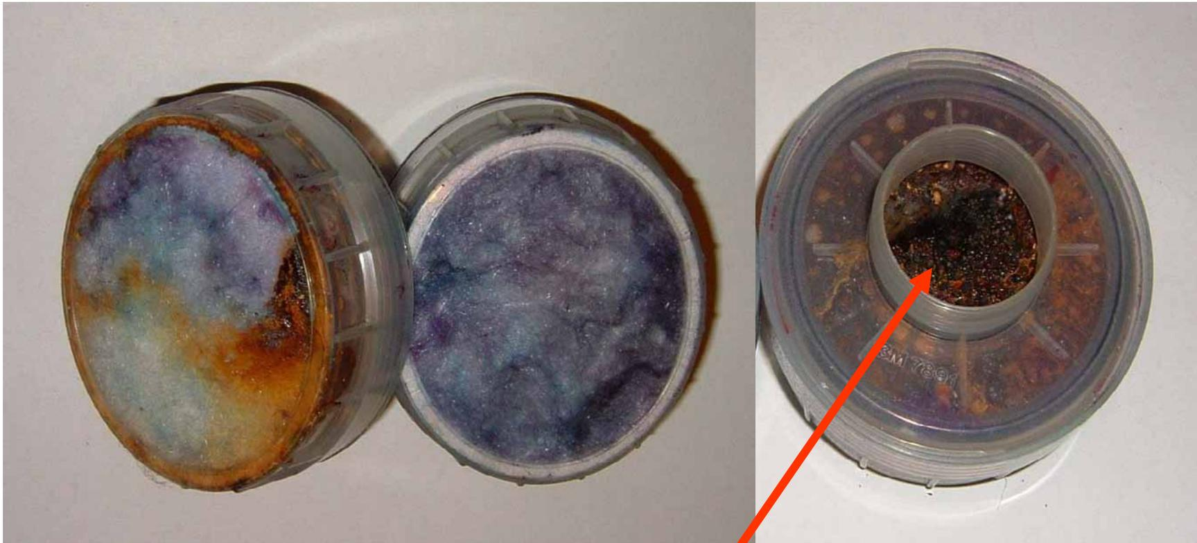
**Inside the normal white surface was replaced with dark brown, crusty material approximately 1/8<sup>th</sup> to 1/4 inch thick.**
