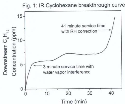
Fig. 1: Cyclohexane service life testing was performed at 1000 ppm  $C_6H_{12}$ , 80% RH, and 100 lpm using an infrared spectrometer downstream detector per CET-APRS-STP-CBRN-0301. Water vapor interference caused a 38 minute loss in service time.
