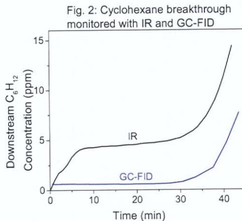
Fig. 2: Cyclohexane service life testing was performed at 1000 ppm  $C_6H_{12}$ , 80% RH, and 100 lpm using a GC-FID as well as an IR spectrometer. The initial leak seen in the IR as cyclohexane is not confirmed by GC-FID.
