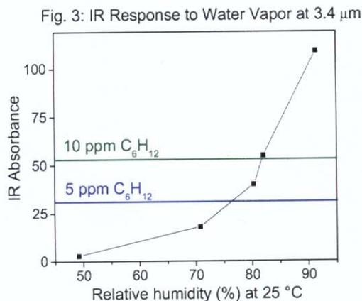
Fig. 3: The IR response to clean air at varying RH. The IR was set to 3.4 micron wavelength, as called out in CET-APRS-STP-CBRN-0301.
