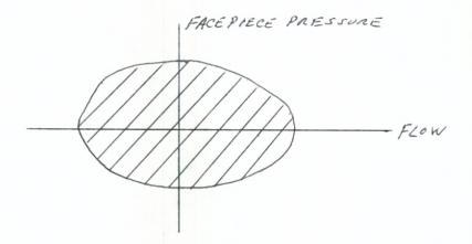
Where an X-Y Plot of breathing volume (flow) vs. face piece pressure is measured, the area within the loop is work of breathing imposed on the wearer by the SCBA. The work of breathing could be measured at 40 and 100 lpm and those values along with protection factor would then be marked on the approval label of the SCBA.
