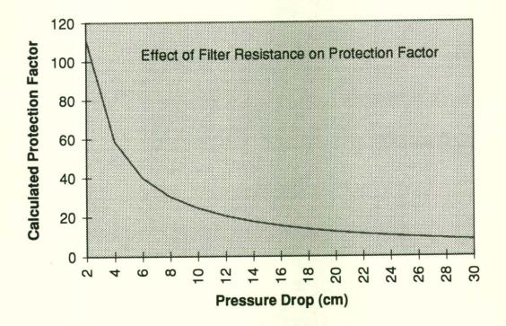
To avoid increased leakage which may result from increasing pressure drop, NIOSH could lower the required filter efficiency for the Type C filter from 95 to 90%, and Type B respirators from 99% to 95%. This reduction in filter efficiency would actually improve the overall protection factor for the respirator by reducing the amount of "pressure drop" associated with its use.
