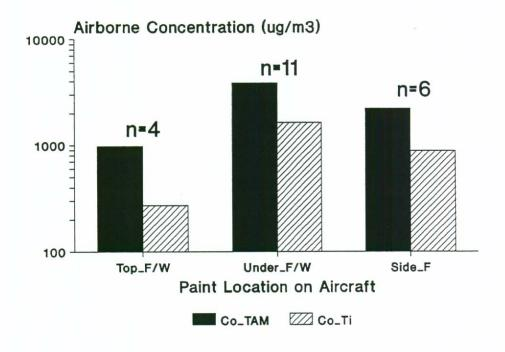
Figure 4 Geometric Mean Concentrations of Total Airborne Mass and Titanium for Application of Top Coat by Location on Aircraft.
