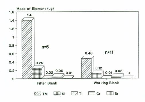
Figure 1 Total Mass and Mass of Various Elements Found on Working Blank and Filter Blank Samples.
