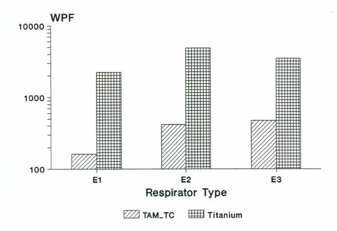
Figure 11 Geometric Mean WPF Measurements for Application of Top Coat Based on Total Airborne Mass and Titanium by Respirator Type.
