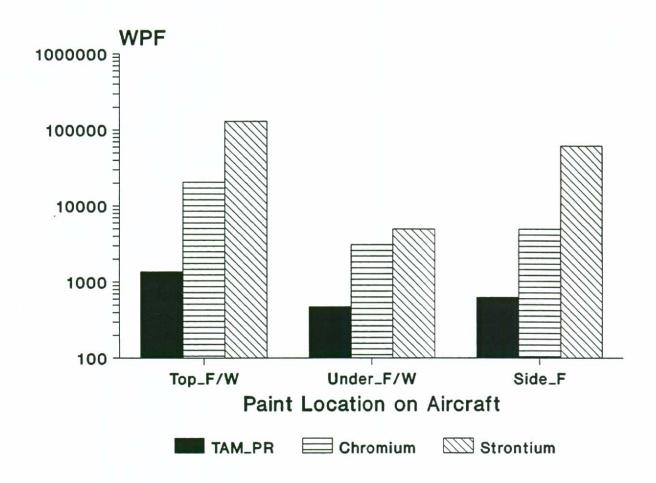
Figure 8. Geometric Mean WPF Measurements for Application of Primer Based on Total Airborne Mass, Chromium, and Strontiumm by Location on Aircraft.
