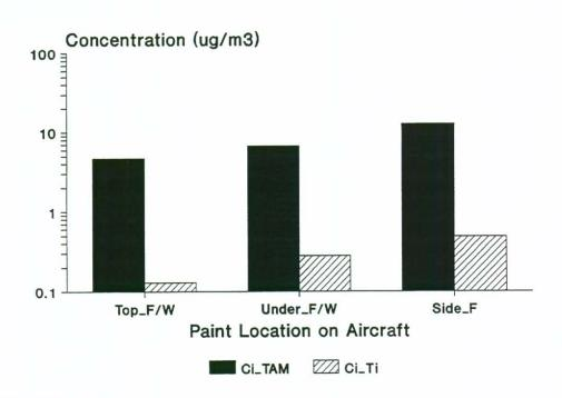
Figure 7. Geometric Mean In-Facepiece Concentrations of Total Airborne Mass and Titanium for Application of Top Coat by Location on Aircraft.
