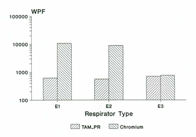
Figure 10 Geometric Mean WPF Measurements for Application of Primer Based on Total Airborne Mass and Chromiun by Respirator Type.
