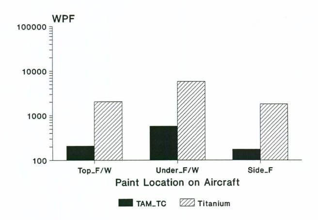
Figure 9. Geometric Mean WPF Measurements for Application of Top Coat Based on Total Airborne Mass and Titanium by Location on Aircraft.
