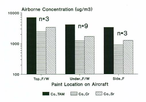
Figure 3. Geometric Mean Concentrations of Total Airborne Mass, Chromium, and Strontium for Primer Application by Location on Aircraft.
