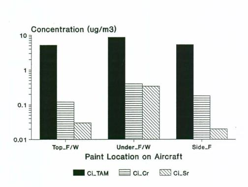
Figure 6. Geometric Mean In-Facepiece Concentrations of Total Airborne Mass, Chromium, and Strontium for Application of Primer by Location on Aircraft.
