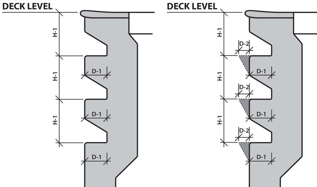
**Figure 4.5.7.4.2: Recessed Step Dimensions: Front View**
