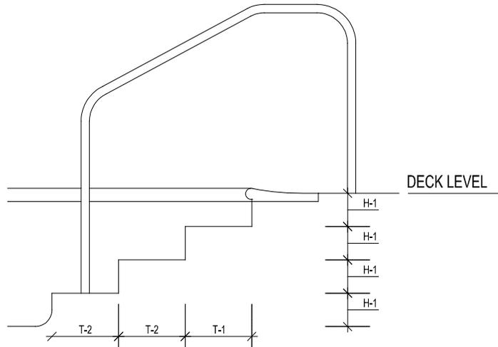
**Figure 4.5.4.5.2: Stair Treads: Front View**
