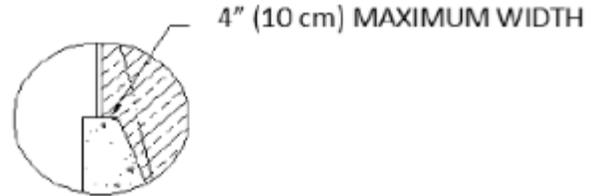
**4.5.17.4.1 Ledge Slope** All structural support ledges and slopes of the wall below shall fall within a plane sloped at a maximum of 1 horizontally in 5 vertically or 11 degrees from the water line down to a water depth of 5 feet (1.5 m). Refer to MAHC Figure 4.5.17.4.
