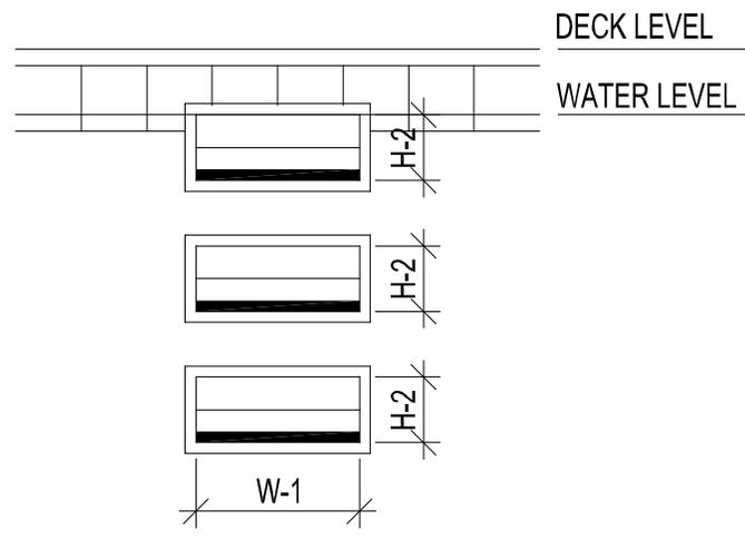
**4.5.7.5 Uniformly Spaced** RECESSED STEPS shall be uniformly spaced not less than 6 inches (15.2 cm) and not more than 12 inches (30.5 cm) vertically along the POOL wall.
