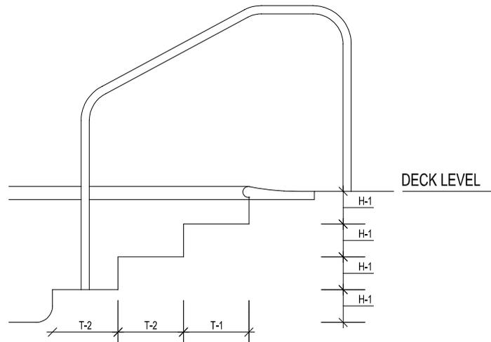
**Figure 4.5.4.5.2: Stair Treads: Front View**
