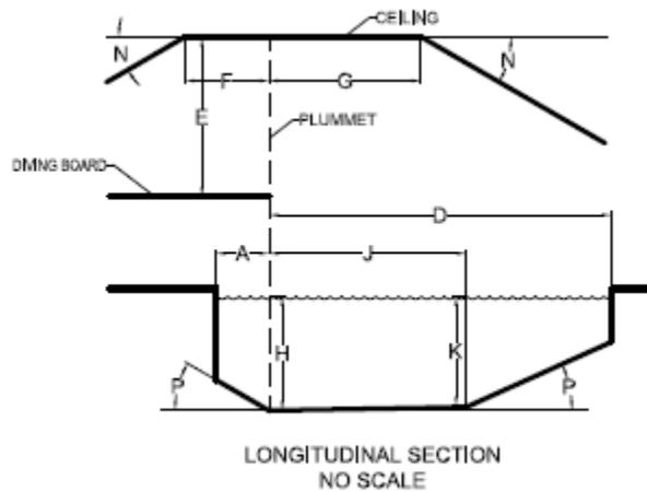
Figure 4.8.2.2.2: Diving Platform Cross Section: Front View
