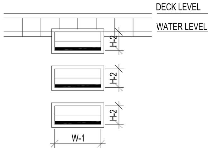
**4.5.7.5 Uniformly Spaced RECESSED STEPS** shall be uniformly spaced not less than 6 inches (15.2 cm) and not more than 12 inches (30.5 cm) vertically along the POOL wall.
