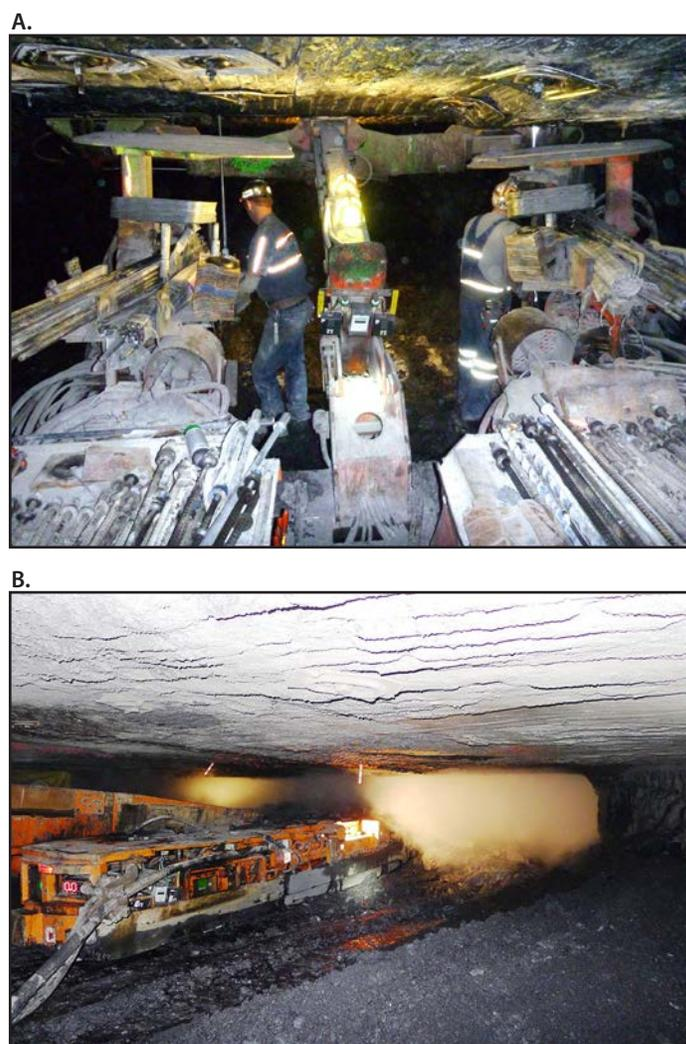
\* A. Two miners use a roof-bolting machine to install the bolts that support the roof of an underground coal mine. B. A continuous miner machine extracts coal from the mine face with a rotating drum.
