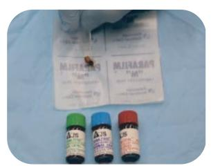
**4.** Perform daily QC testing and recording for the low, normal, and high-range control vials. Place a drop of QC material on a nonabsorbent surface (e.g., a piece of plastic film), then position the cuvette in the center of the drop.
