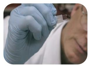
**8.** Inspect the cuvette for air bubbles.
