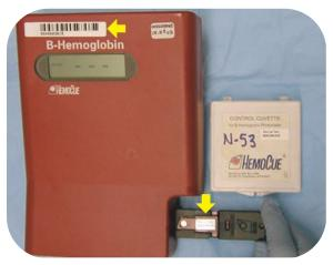
2. Check the instrument for accuracy using the instrument-matched calibration cuvette. For readings outside the specified range, clean the cuvette holder and cuvette with a dry, lint-free wipe. For readings within the range, perform daily quality control (QC) testing.
