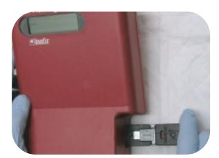
Place the cuvette in HemoCue® instrument. Gently push the holder into the photometer. Record the result.
