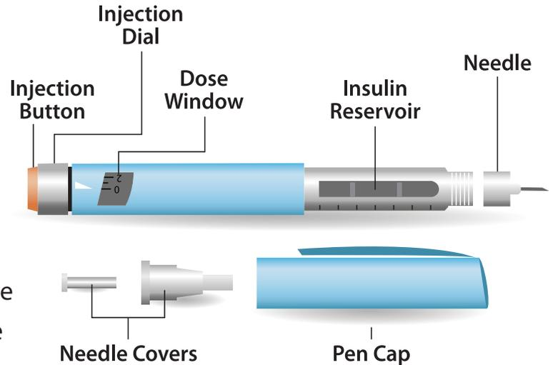
Although invisible to the eye, back flow of blood into the insulin pen can happen during an injection. This creates a risk of bloodborne and bacterial pathogen transmission to patients if the pen is used for more than one person, even when the needle is changed.
