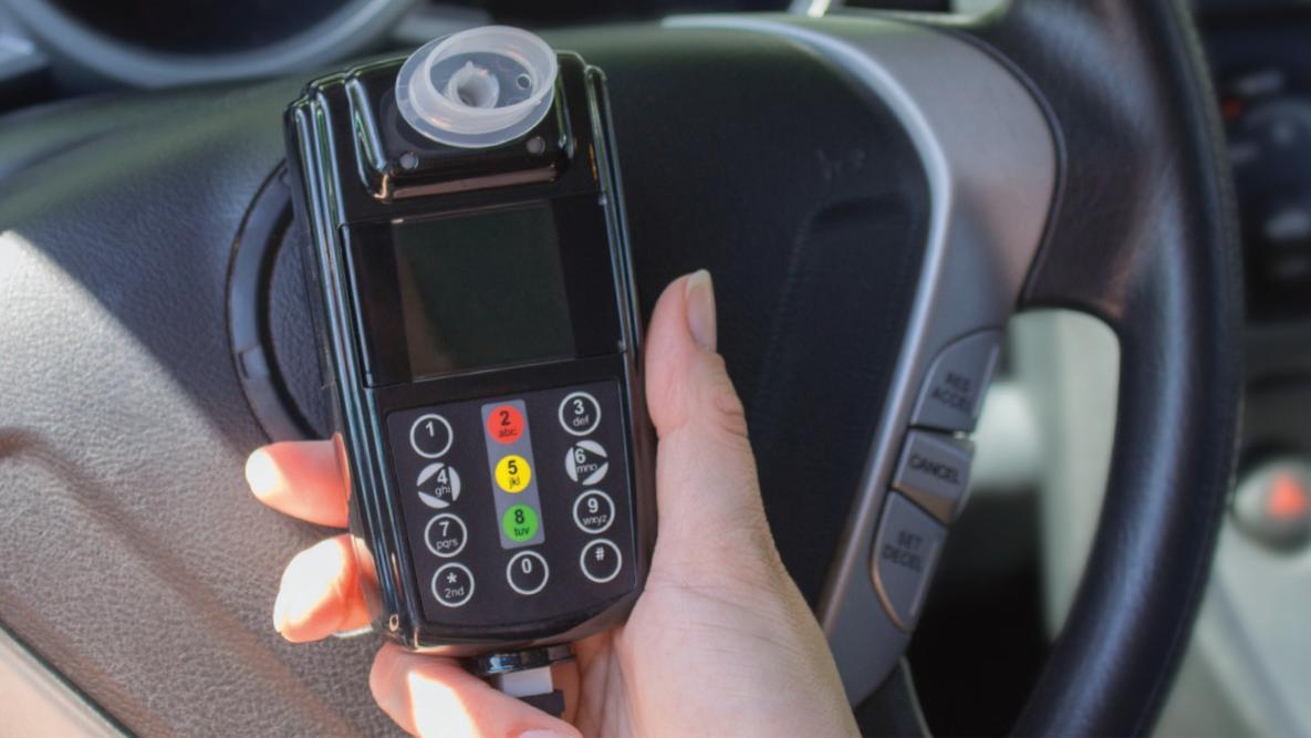
◀ An alcohol ignition interlock is a breath-test device connected to a vehicle's ignition. The vehicle will not start unless the driver blows into the interlock and has a blood alcohol concentration (BAC) below a pre-set low limit, usually .02 BAC.
