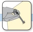
When the nail gets hot, press the point against the mark on the container to make a hole.
