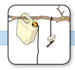
Hang the container by its handle. Hand it high enough so the rope holds the end of the long stick off the ground. Hand the soap near the container.
