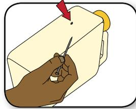
**1** The tippy tap needs a hole for the water to pour out of. The hole should be on the side of the container across from the handle. The hole should be a finger length from the top of the container. Find the spot for the hole and make a mark there.
