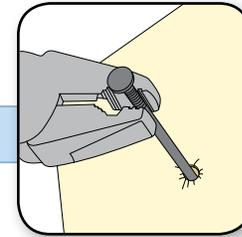
**3** When the nail gets hot, press the point against the mark on the container to make a hole.
