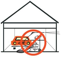
NEVER place pressure washer engines in garage, carport, or other enclosed space during use.
