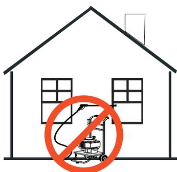
NEVER place pressure washer engines near open windows, doors, or vents during use.
